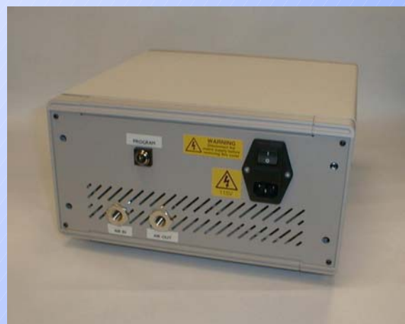
Rear view of Air Leak Test Unit
